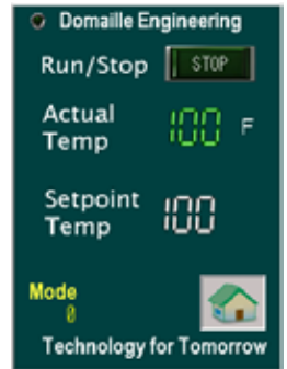
FIG 15. Actual Temp turns GREEN when within alarm tolerance of set point.
